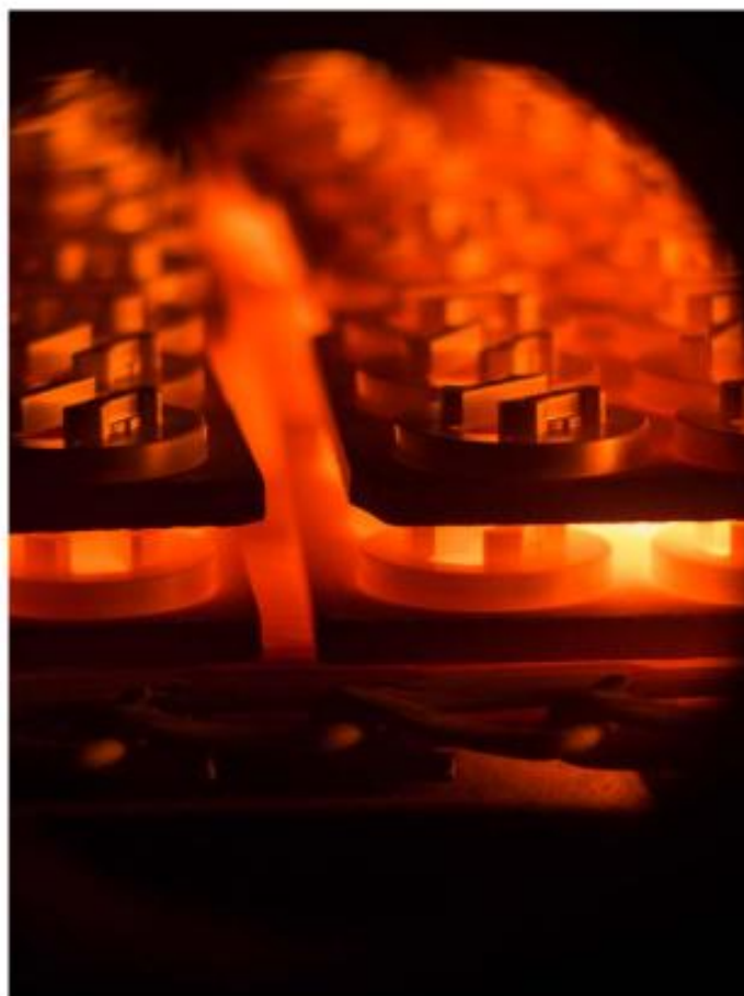
Fig. 3 Sintering of PM parts (Courtesy Gevorkyan)
